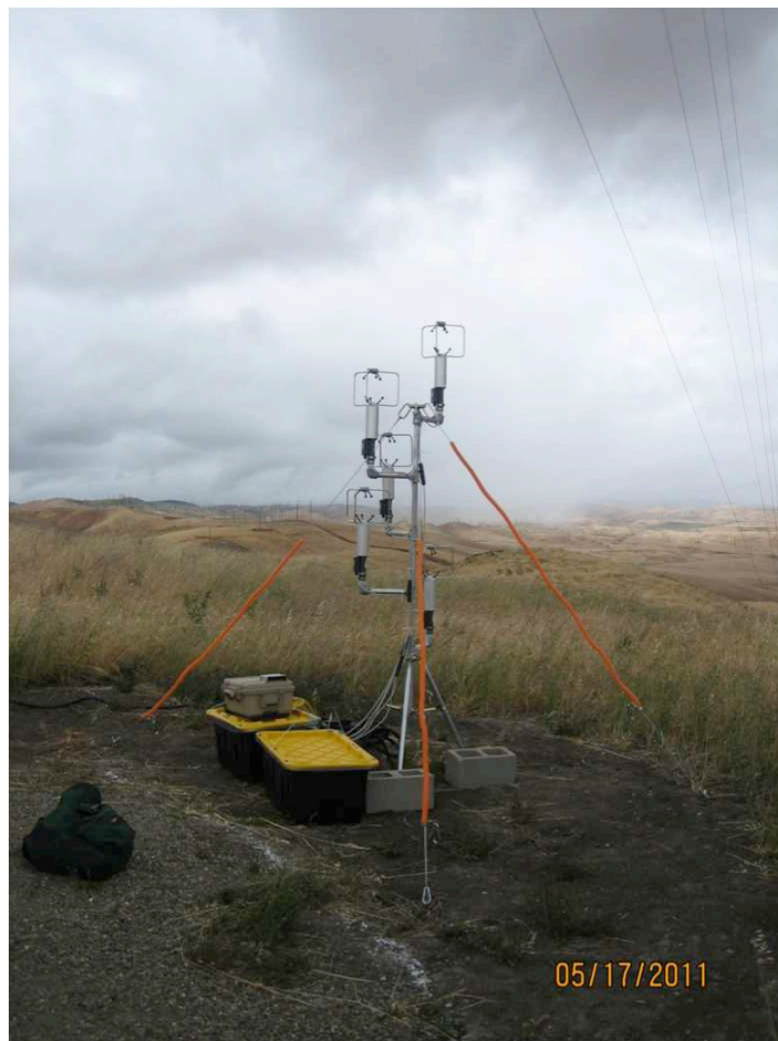
Google's anemometer array for measuring surface wind characteristics
