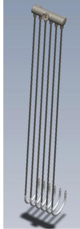
**Receiver tubes (each 4 meters long and with a 32mm OD); curves at bottom are to mitigate thermally induced stresses and strains**
