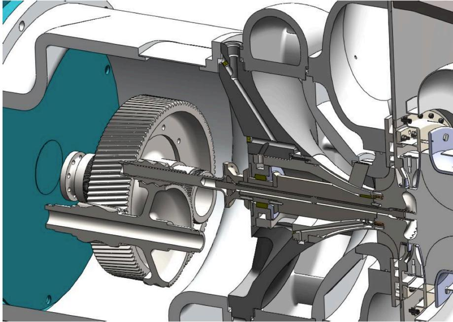
**Gearbox configuration. Generator is on left, HP spool on right**
