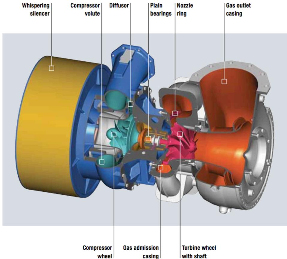
**Cutaway view of low-pressure spool - an [off-the-shelf turbocharger](#) made by MAN Diesel & Turbo SE**
