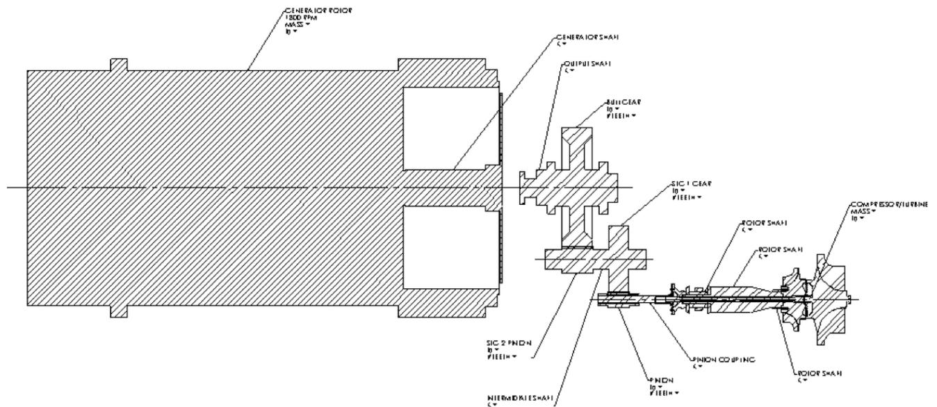
**High pressure stage layout: generator rotor, gearing, and spool**
