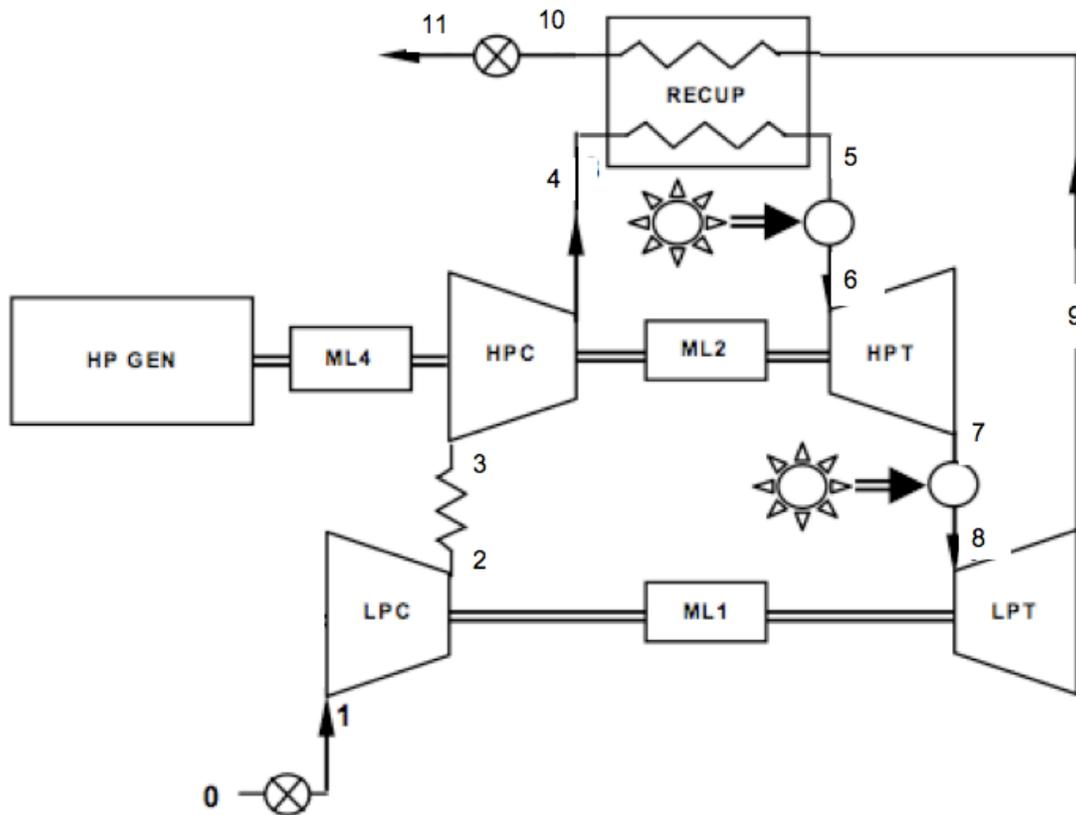
**Modified engine configuration (A1) with a single constant-speed generator**
