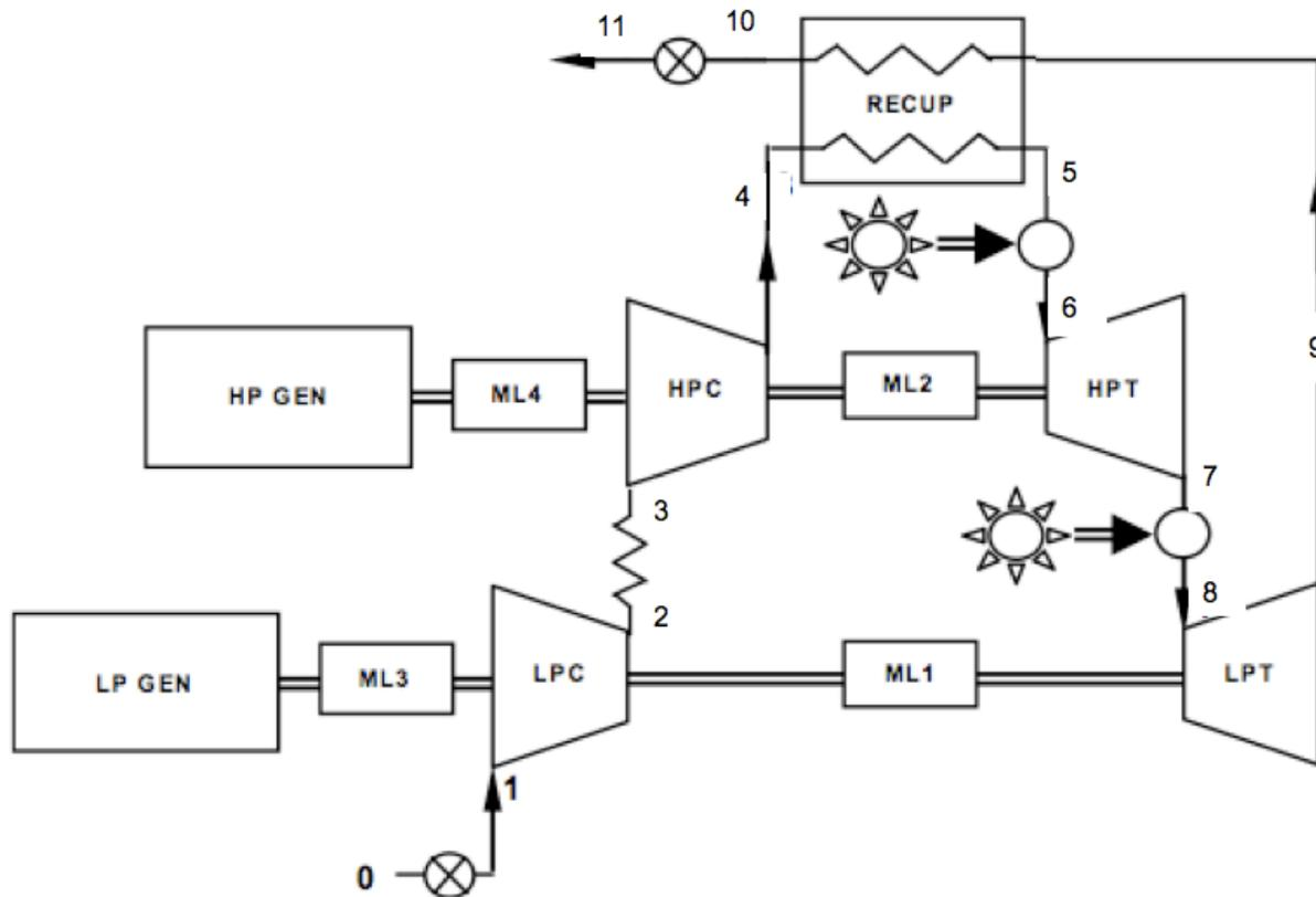
**Initial engine configuration, an ICRR cycle (intercooled, recuperated, reheat)**
