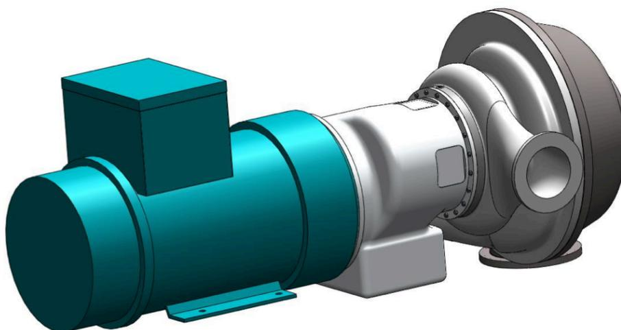
**High pressure stage assembly. From left: generator, gearbox, and HP spool**
