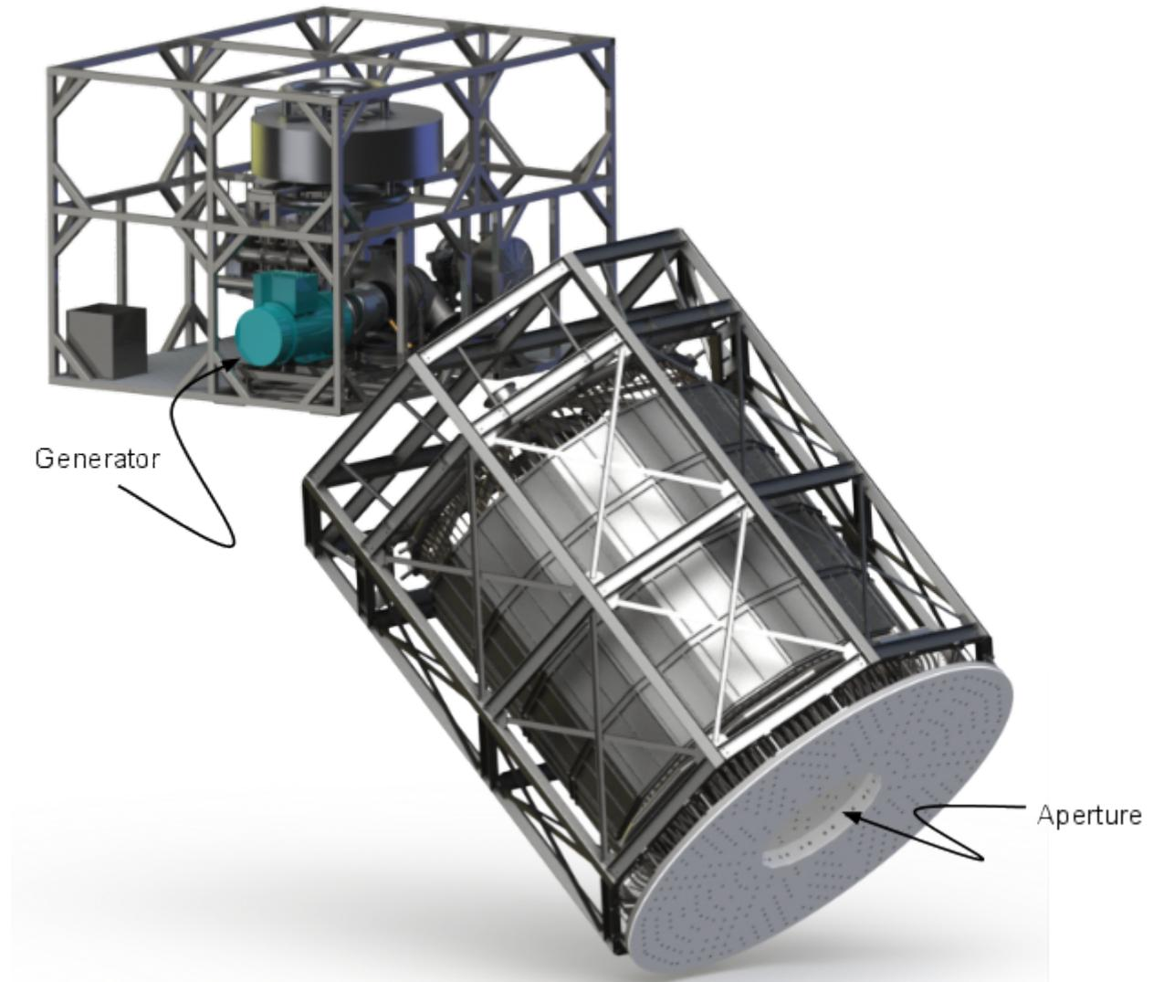
**Fully assembled engine and receiver (aperture diameter is 1.5 meters, and overall receiver is roughly 6.5 meters long)**
