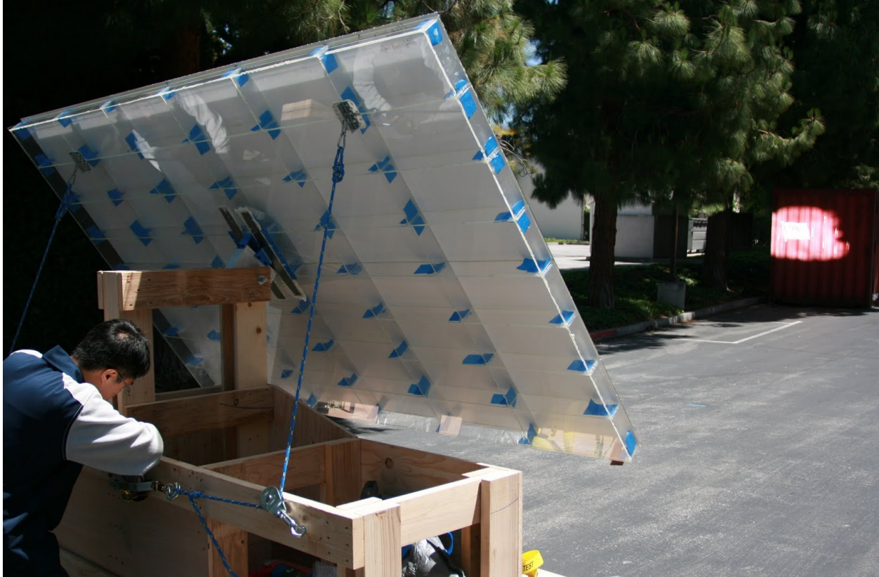
Heliostat reflector mounted on a test platform
