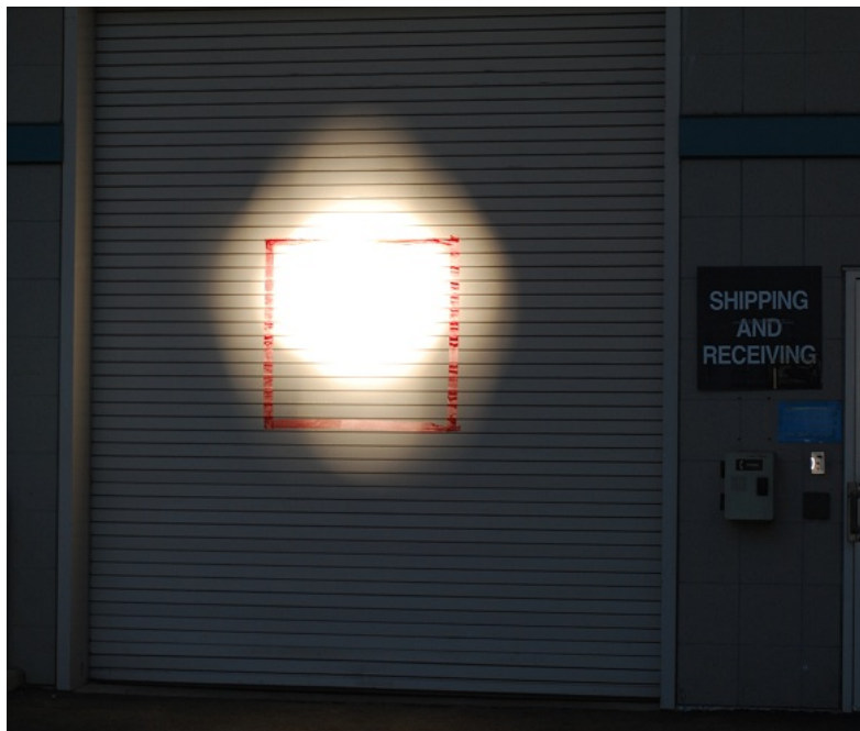
Solar reflection from a 2m x 3m prototype mirror on a 1m x 1m target, showing a bright 1m diameter focused spot but also some light spillage. Improvement may be required depending on the target requirements.
