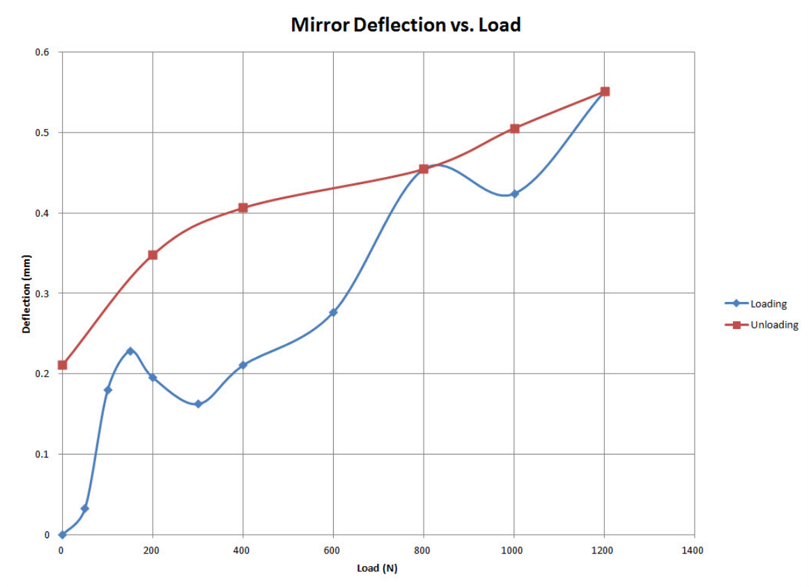
Reflector stiffness testing
