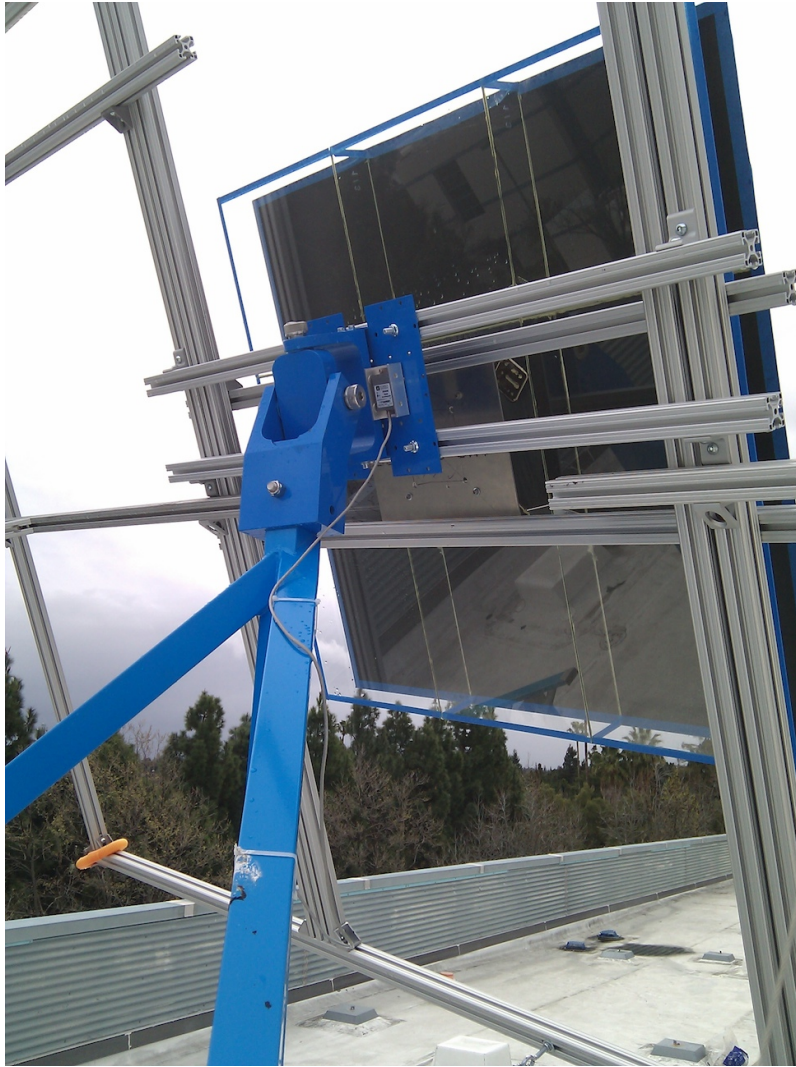
Close-up of a prototype heliostat with a 3-axis accelerometer mounted (the small gray box). Note that this prototype does not have a mirror angle offset.
