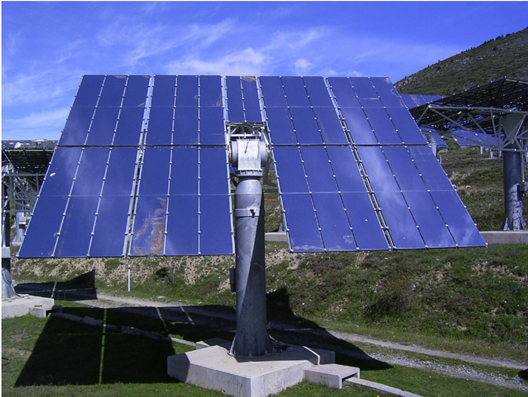
An azimuth mounted heliostat at the THÉMIS experimental station in France (Image courtesy of Wikipedia)
